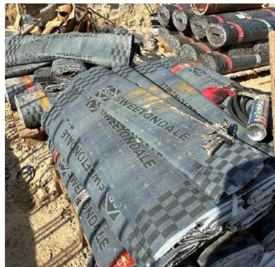
Figure 5. Bitumen-rubber primer and waterproofing film.
